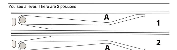
1 = below - release with pressure at point A upwards
